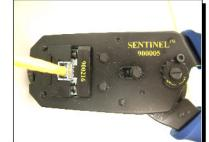
6. Pull load bar forward flush with ends of conductors.
