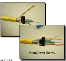
5. Cut Conductors to .160 /.180 inch from load bar as shown.
