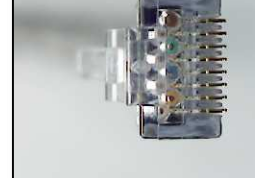
15. Bottom conductors fully into their openings.
