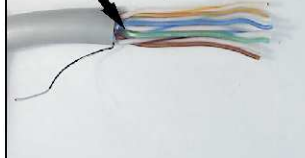
7. Straighten wires. Maintain twists in this area. Do not untwist into jacket.
