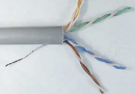
6. Remove pair divider. Organize pairs into proper order.
